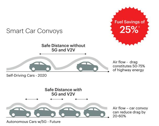
5G vehicle-to-vehicle communications (V2V) could allow lead cars to communicate hazards to following cars, increasing reaction time and
