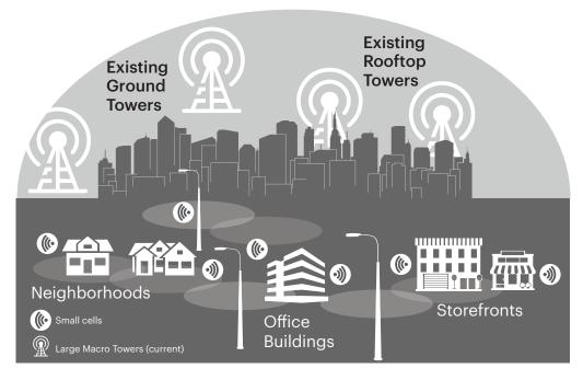
Existing towers will provide coverage for miles, while small cells will support the increased needs of a Smart City.
