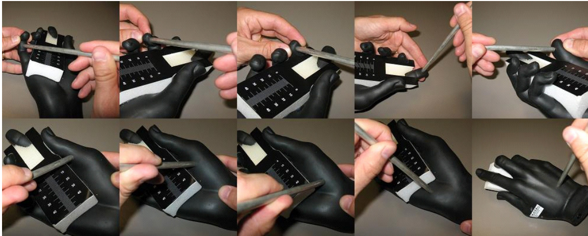
FIGURE G-1 TEN LOCATIONS OF DIELECTRIC MEASUREMENTS AT THE BRICK HAND SURFACE
