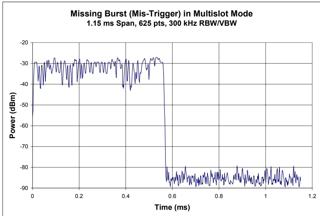
FIGURE D-12 BAD 8-PSK MULTISLOT TRACE RESULTING FROM MIS-TRIGGERING
